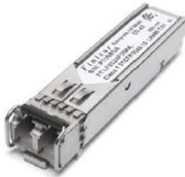
Fig. 2.2: The pluggable transceiver component of A3818
